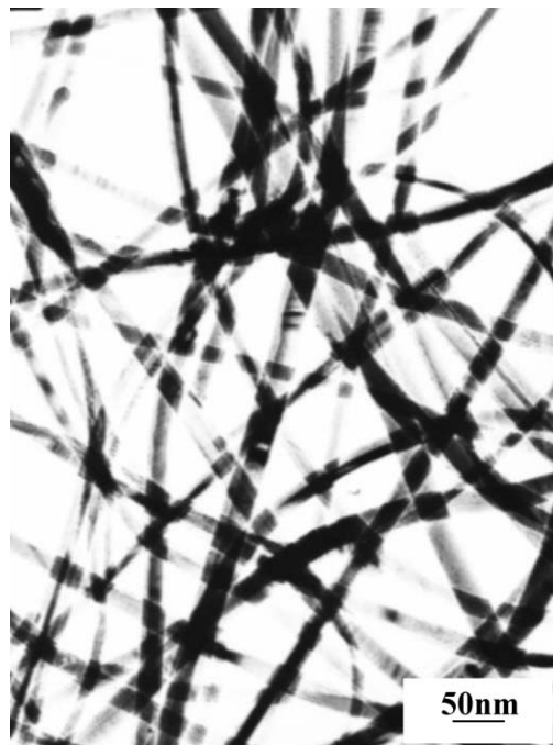
Figure 4 A TEM image of the \beta -SiC nanowhiskers.
